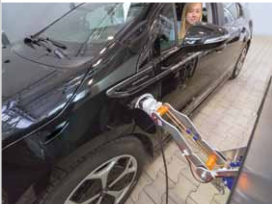
Fully automatic charging station
